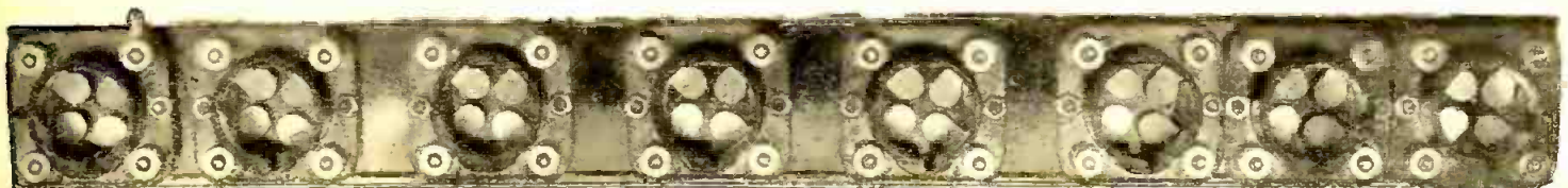
The socket strip for the simplified portable super-heterodyne, showing one filament lead and method of binding lugs for other filament lead.
